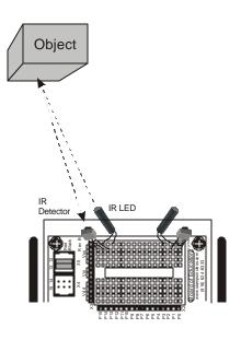
Figure 5.1: Object detection with IR Headlights.
