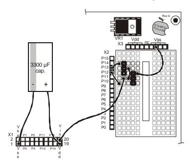
Figure D.2: Servo Port Wiring.
