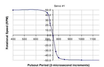
Figure 1.29: pulsout period vs. rotational speed for servo.
