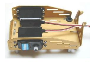
Figure 1.8: Servos mounted on chassis.
