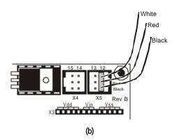
Figure 1.15: Servo ports on the BOE Rev B (a) before, and (b) after plugging in servo port 12.
