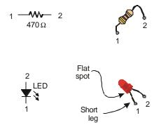
Figure 3.6 Extra parts for testing the whiskers.
