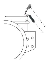
Figure 6.3: IR LED adjustment for edge detection.
