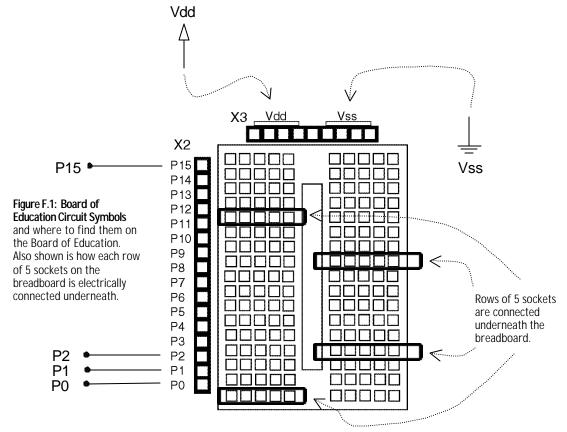
Next, the ground symbol is used for Vss. This is the reference terminal for taking measurements, and it's considered to be 0 volts compared to all other voltages on the Board of Education. The four sockets for connecting jumper wires to Vss are along the top of the breadboard to the right.
