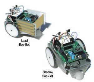
Figure 6.5: Lead and shadow Boe-Bots.
