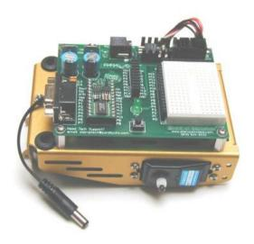
Figure 1.14: BOE attached to chassis.
