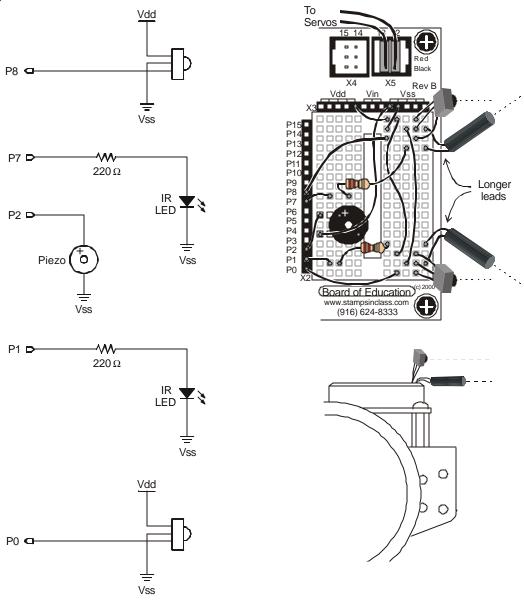
(b) wiring diagram.
