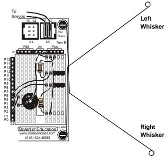
Figure 3.3: Whiskers wiring diagram.
