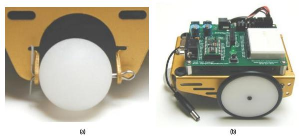
Figure 1.17: (a), Tail wheel mounted on Boe-Bot chassis, and (b), front wheel mounted on servo output shaft.
