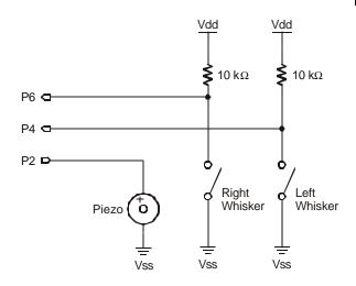
Figure 3.4: Whiskers Schematic.
