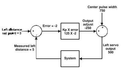
Figure 6.4: Boe-Bot proportional control block diagram.
