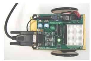
Figure 1.20: (a), Serial cable connected to comport,
