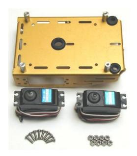
Figure 1.7: Servos and mounting hardware.
