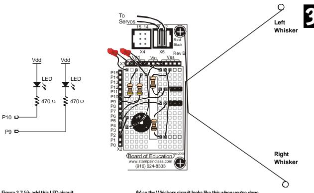
Figure 3.7 (a): add this LED circuit,
