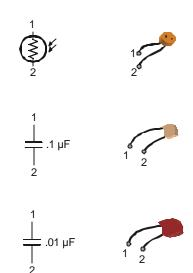
Figure 4.2: Photoresistor and capacitor circuit symbols and parts.
