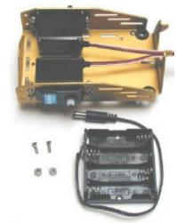
Figure 1.9: Battery pack and mounting hardware.
